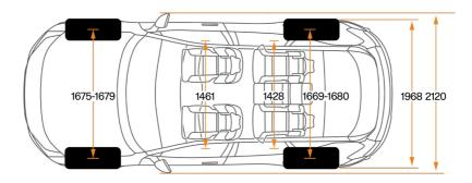
Dimensions (mm): L-4900 mm H-1614 mm W-2120 mm Wheelbase (mm): 2985 mm Tyre specs: 21" 265/45 295/40 – 22" 265/40 295/35 Luggage volumes front/rear (liters): 32 L / 597 L
