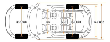
Dimensions (inches): L-192.9" H-64.1" W-83.2" Wheelbase (inches): 117.5" Tyre specs: 21" 265/45 295/40 – 22" 265/40 295/35 Luggage volumes front/rear (cubic feet): 1.1 cubic feet / 17.1 cubic feet
