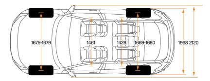
Dimensions (mm): L-4900 mm H-1618 mm W-2120 mm Wheelbase (mm): 2985 mm Tyre specs: 21" 265/45 295/40 – 22" 265/40 295/35 Luggage volumes front/rear (liters): 32 L / 597 L
