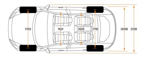
Dimensions (mm): L-4840 mm H-1534 mm W-2139 mm
